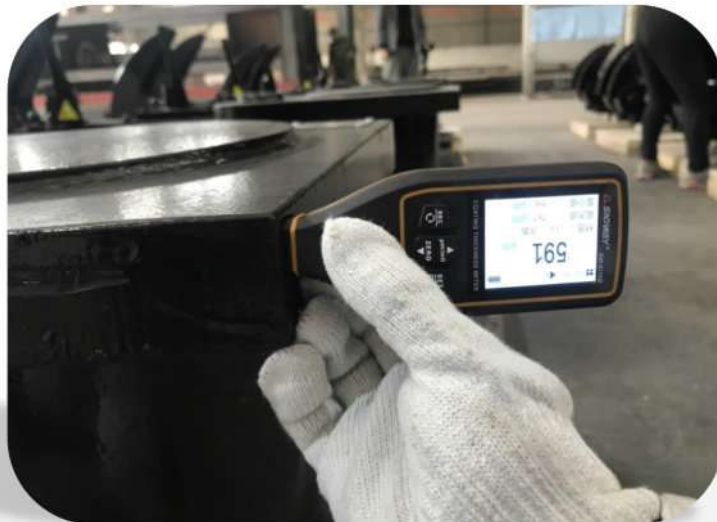
Coating Thickness Checking
